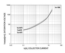
Figure 3. Base-Emitter Saturation Voltage
